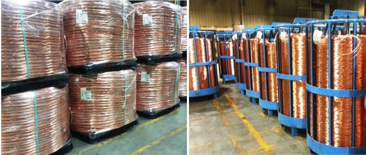
**Figure 1.** Copper Rod (left) and Copper Wire (right) Made at Essex
